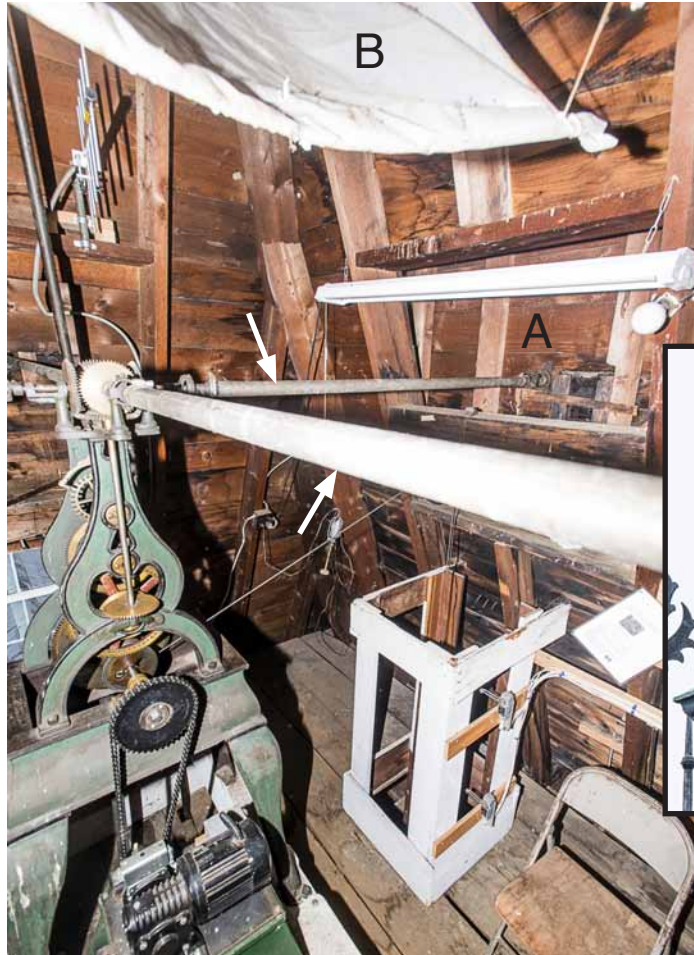
Photo 92: Top level of clock tower with clock mechanism on lower right. The arrows point to the shafts linking the clock movement to the clock faces. "A" marks the interior of the northerly clock face. "B" marks a sheet of plastic that has been set up to protect the clock mechanism from occasional leaks from coming the top of the tower.
